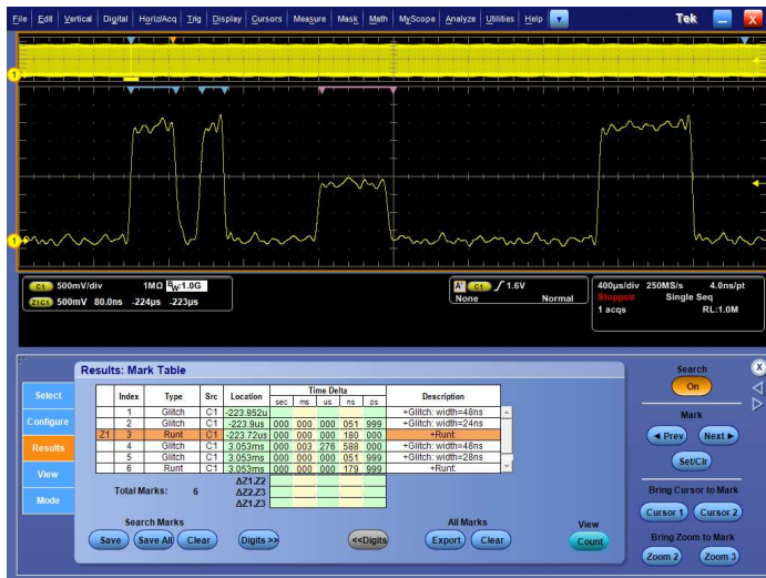
Search - Results of an advanced search for a runt pulse or a narrow glitch within a long waveform record.
